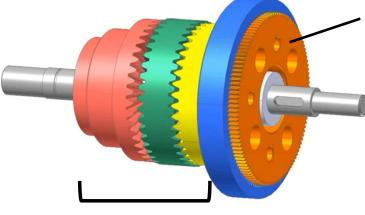
Sun gear holds its posture (Eccentric mechanism holds it)
