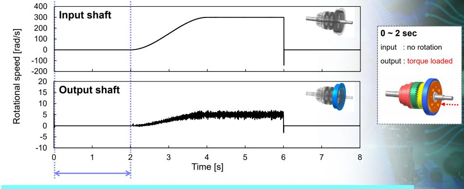
The rotation speed is 0 for both input and output because rotation is not transmitted from the output shaft (it was locked)
