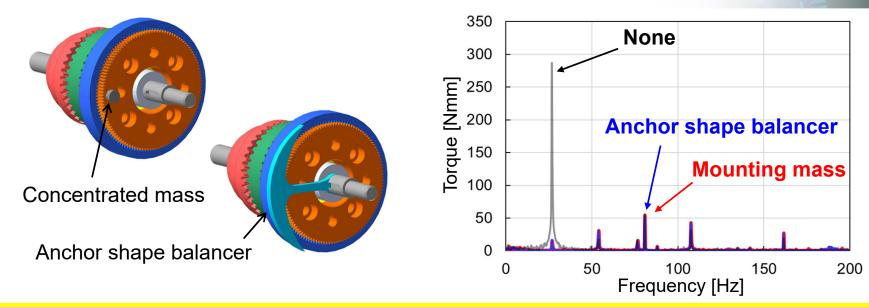
By mounting mass, vibrations in primary rotation order can be reduced
